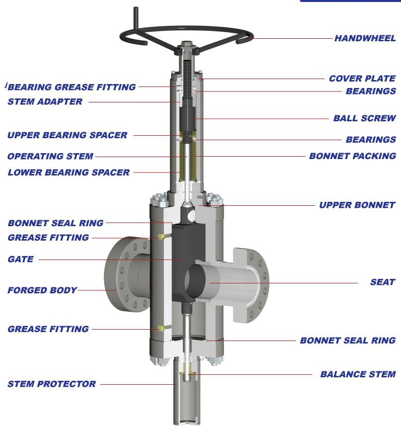
j) Valve bonnet / ball screw housing (where applicable) equipped with grease port(s) and fitting(s) for bearing lubrication
