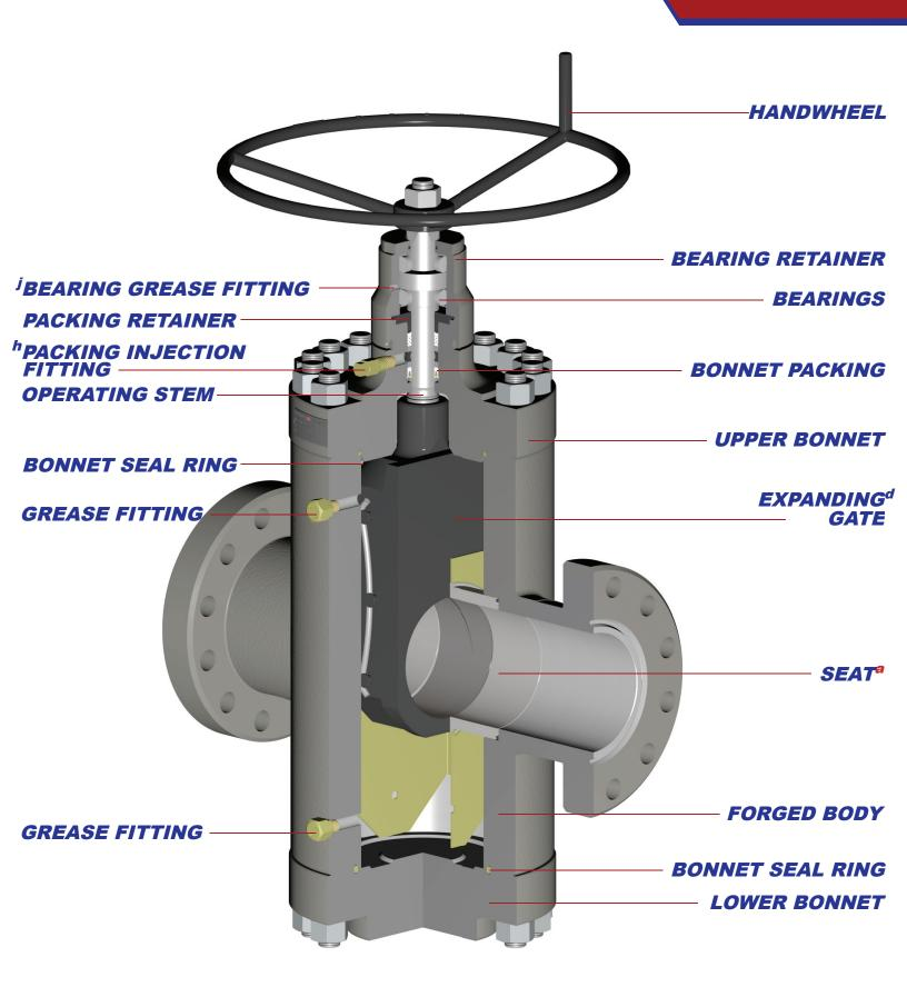
a) Equipped with a non-sealing seat on the upstream side. See engineering note titled "Model FM4 & Model FM4 RC" for details.
